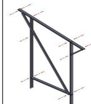
Assemble the individual support structure sections as per the drawing. The sections are delivered in pieces according to the structure design with the members loose. Secure all joints firmly on both sides with the self-drilling screws provided using an electric drill with appropriate screw bit.
