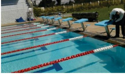
Anti-wave racing lane dividers made from 150mm diameter UV stabilized high density polyethylene discs assembled on stainless steel
