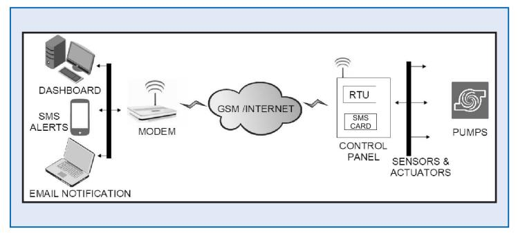
iDAYLIFF is an innovative remote control system designed for the control and monitoring of water pumps. It is available as an option on any DAYLIFF pump control panel and provides users with specific information about the operation of their pumping system.
