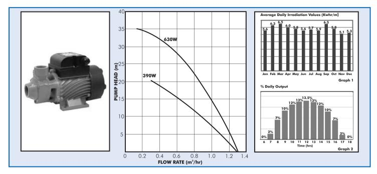
The DAYLIFF DDPS 60 are solar booster pumps suitable for water transfer in small scale applications where grid power is unavailable. It is constructed of cast iron pump body, aluminium motor body, peripheral brass impeller and silicon carbide mechanical seal.
