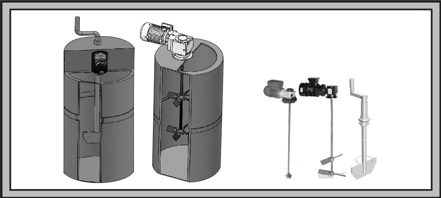
DAYLIFF chemical tanks are specially designed for use in dosing applications of various concentrate chemicals. They are made from strong corrosion resistant GRP and are available in various sizes according to applications. All are provided with a reinforced top to support a dosage pump mixer, an inspection/filling cover and a graduated chemical volume scale. A variety of dosage pumps are available to suit the dosage requirement.
